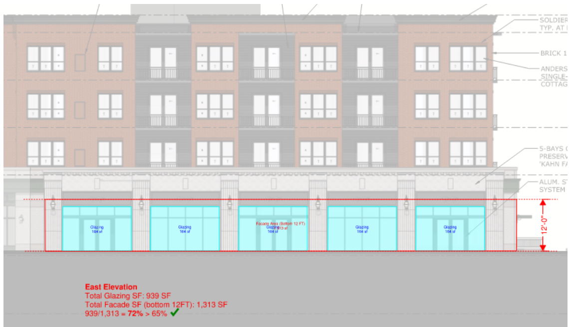
Figure 7: Example Ground Floor Glazing Calculation
